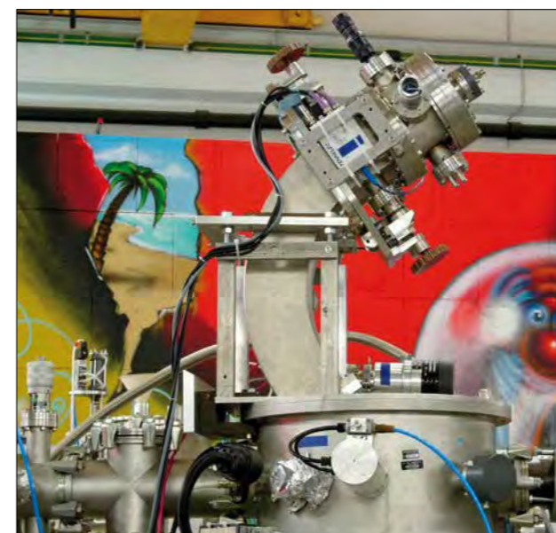
Fig. 1: High resolution RBS setup showing the scattering chamber and the cylindrical electrostatic analyzer providing a depth resolution of < 2 nm.
