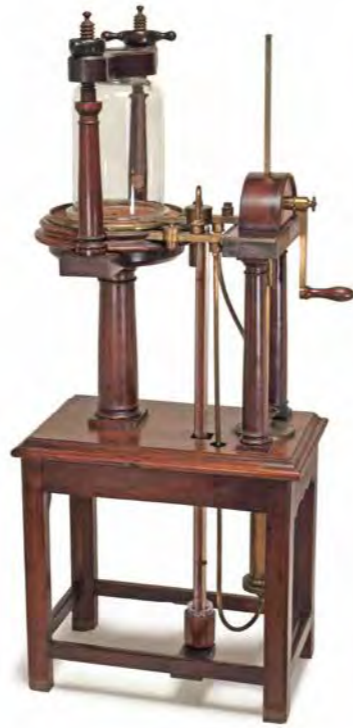
Fig. 2: Vacuum pump (manufactured by Naire and Blunt, London 1782). It was the most expensive piece of equipment in Lichtenberg's collection, reaching a vacuum of 0,5 mbar (Quelle: Sauer Marketing).
