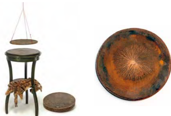
Fig. 3: Electrophorus and cat fur on the left at around 1780. With the tin foil coated wooden plate the charge could be separated and impressive electric sparks up could be generated. Lichtenberg figure for a positive charge on the right (Quelle: Sauer Marketing).
