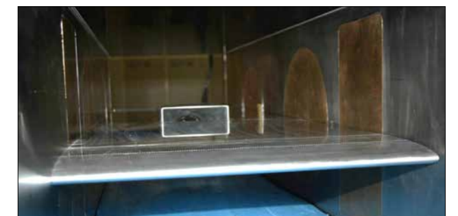
Fig. 2: Generic intake on a flat plate in the cryogenic wind tunnel KRG of the German-Dutch Wind Tunnels DNW.
