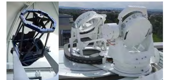
Fig. 5: At the Institut für Astrophysik, we are operating two telescopes: 50cm Cassegrain nighttime telescope (left), and a 50cm Siderostat (right) for daytime observations of the Sun
