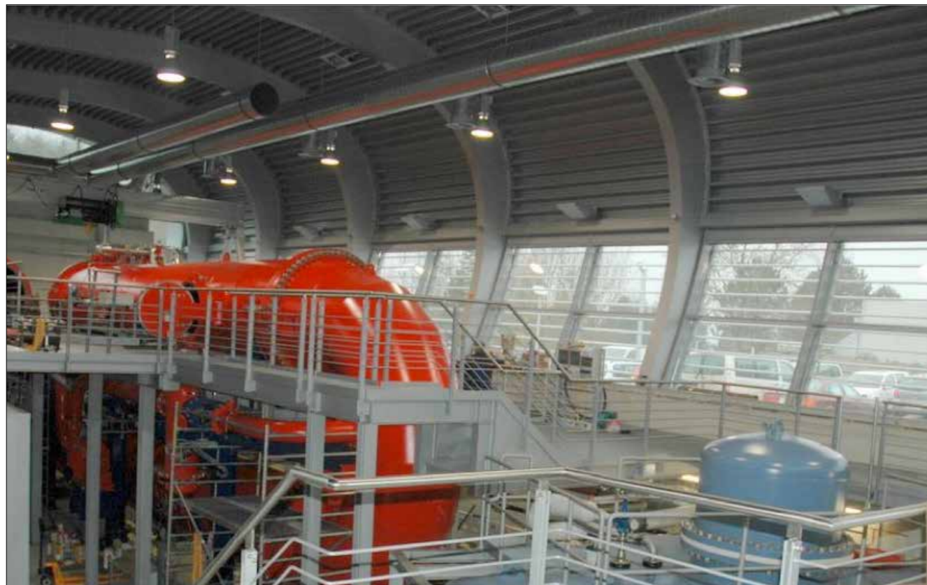
Fig. 2: Göttingen Turbulence Facility. The red tunnel is 18m long and 6m high. The blue “submarine” has a 2.5 m diameter and is 5 m long, the turret is 4m high. The vessels can be filled up to 20 bar with SF 6 gas.
