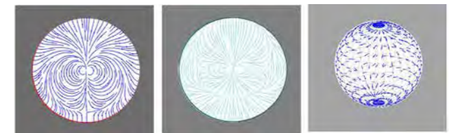
Fig 4: From left to right: directions of active polar molecules within a droplet filled with a viscous liquid are shown in a cross section (left); they create a force field (middle), which sets the liquid into motion. The active surface velocity (right) leads to self-propelled motion of the droplet, if it immersed in water.
