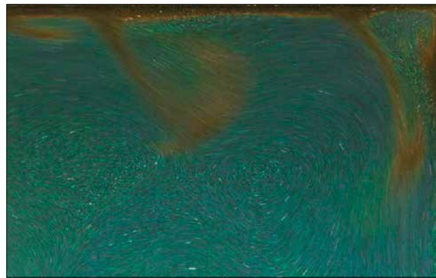
Fig. 4: Picture of eddies and plumes detaching from a cold plate at the top of the picture in convecting water. Particles filled with thermochromic liquid crystals have been suspended in the water. The liquid crystals change color with temperature, and the velocity field is visible as streaklines in this photograph with a 1 s exposure time.
