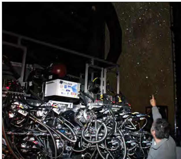
Fig. 2: The Multi Unit Spectroscopic Explorer at the Very Large Telescope. (credit ESO)
