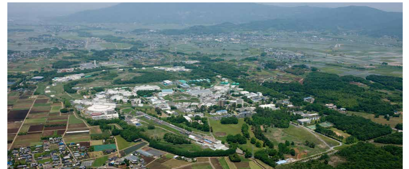
Fig. 1: Aerial view of the KEK site located about 70 km from Tokyo with Mount Tsukuba in the background. The 400 m long electron/positron linear accelerator and the buildings above the collider ring whose circumference is about 3 km can be seen.
