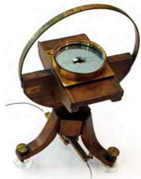
Fig. 6: Weber's instruments to measure the magnetic field generated by the circular current loop from 1837. With the Tangenten-busssole (Bussole = compass), sensitive deviations of the needle could be determined thus it was the first practical instrument to measure the magnetic field generated by the current through the wire loop. The wiring can be seen at the bottom.
