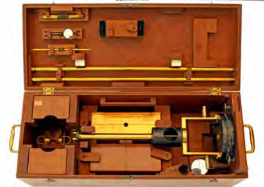
Fig. 5: Transportable magnetometer from Weber (manufactured by Meyerstein Göttingen, 1839). It was motivated by Alexander von Humboldt to map the earth's magnetic field component, which was deduced from 100 experimental stations all over the world and printed in Gauß' and Weber's atlas of the earth's magnetism.
