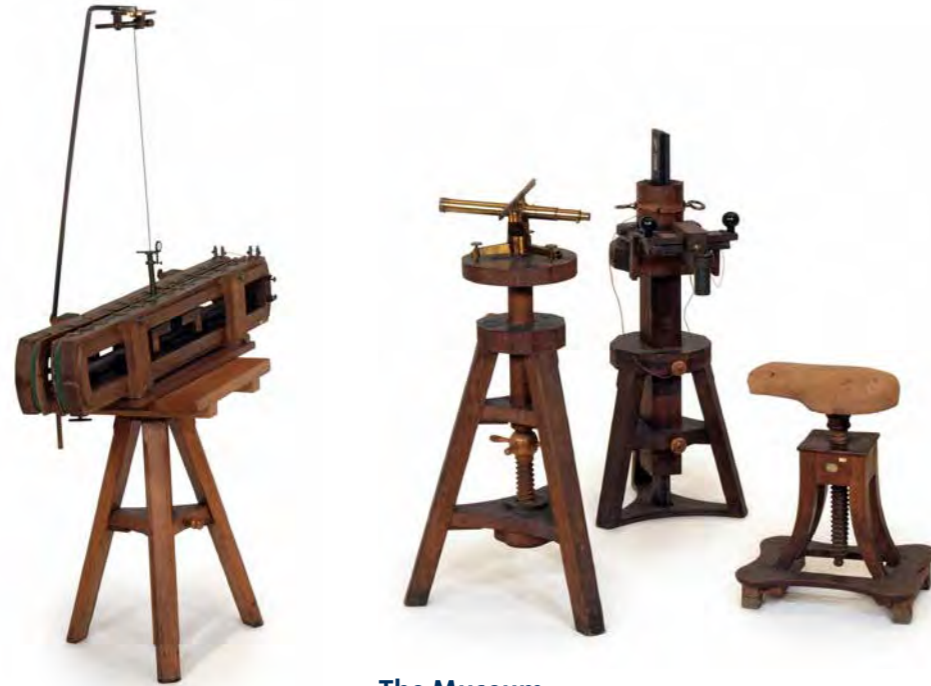
Fig. 7: Gauß-Weber telegraph as shown at the world exhibition in Vienna 1873 (Quelle: Sauer Marketing).
